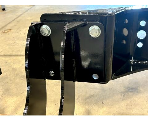
Step 3: Attach this to outside of track frame (see picture below). Use 20mm by 90m bolts to mount this to frame.
