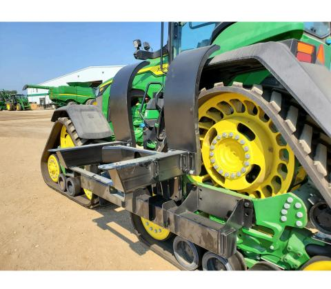
Step 6: Align the tubing and tighten the 5" x 7" steel brackets together with step plate. Attach with 4 - 3/4" x 8 1/2" bolts, with 8 washers, and 4 nuts. See next picture.
